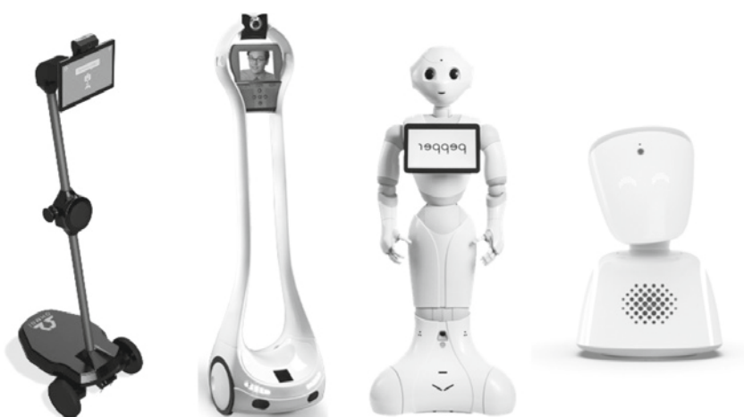
Figure 2. Different telepresence systems (from left to right): Ohmni (©Ohmnilabs), VGo (©VGo Communications), Pepper (©Softbank Robotics), Avatar AV1 (©No Isolation).
